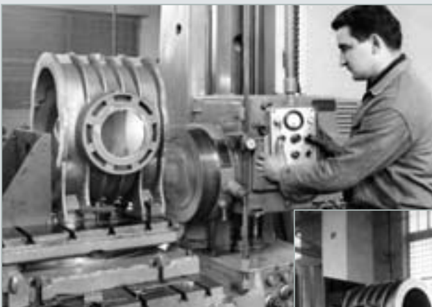
ROR The 60s: ROR blowers casing - sides manufacture
